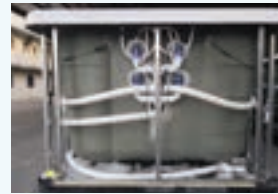
Galanised Steel frame with side and seat supports
